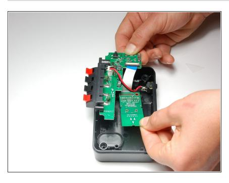
Flip over the motherboard and wireless audio module chip.
