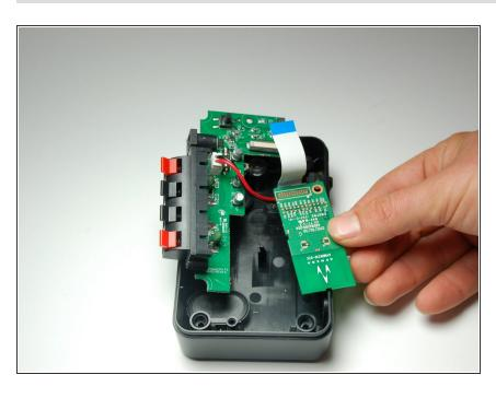
Using your fingers, pull the ribbon wire out from the black retaining flap in order to completely disconnect the wireless audio module chip.
