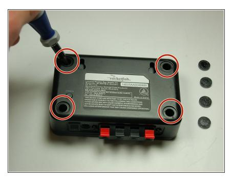
Use a Phillips #1 screwdriver to unscrew the four 12 mm screws on the bottom of the device.
