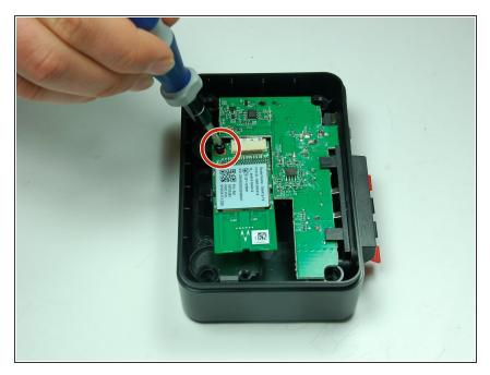
Use a Phillips #1 screwdriver to unscrew the 10 mm screw, securing the wireless audio module chip.
