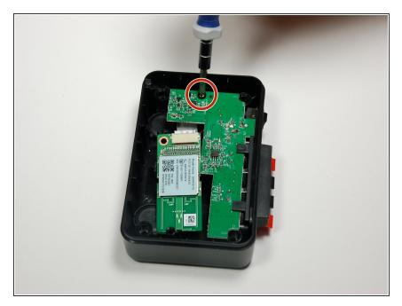
Use a Phillips #1 screwdriver to unscrew the 10 mm screw, securing the motherboard.
