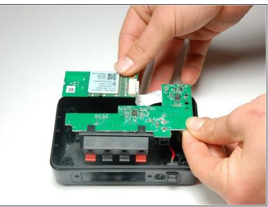
Using both thumbs, push the front speaker input terminal back towards the inside part of the device.
