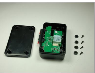
Flip the device over and remove the top casing from the sender.
