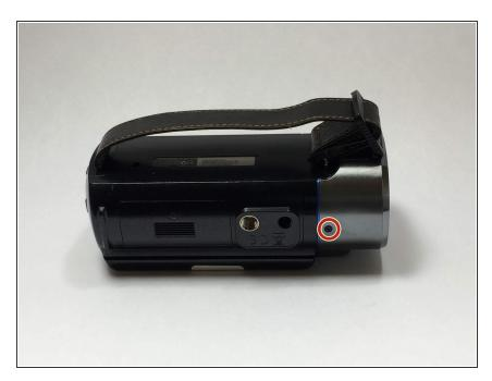
Remove the 4 mm screw on the underside of the camcorder near the tripod mount.
