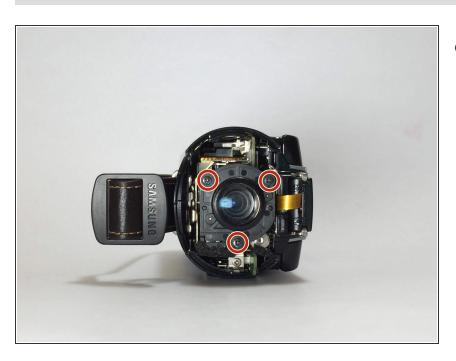
Remove the three 5 mm screws surrounding the lens.
