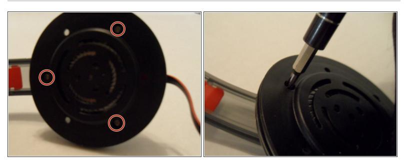
• Use a Phillips #0 to unscrew three 3.4MM screws from the earpiece.
