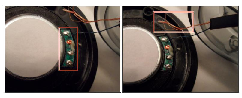
Find the wires connected to the speaker and check if they are intact.
