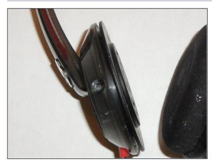
Locate the grooves where the cushion should be located on the earpiece.
