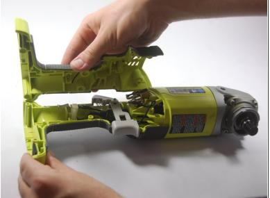
Now that the two halves are unscrewed, lift up the top half.
