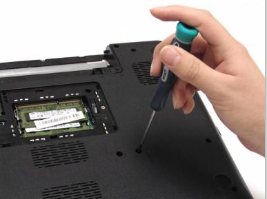
Close cover and turn laptop over. Locate and remove the four hard drive screws.
