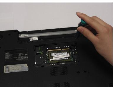
• Locate and remove the 2.5 mm x 5 mm screw on the upper right hand side of the compartment.
