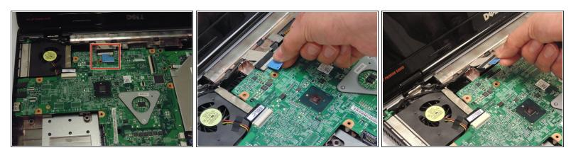
Turn laptop over and open it. Locate and unplug the LCD Cable.
