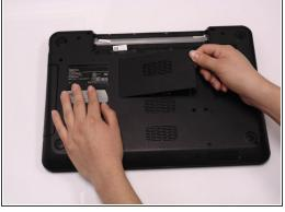
Locate the RAM compartment and the screw on the right hand side. Remove the cover.
