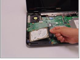
Lift and remove the hard drive.
