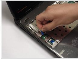
• Locate the palm rest cables. Lift the black levers and unplug the blue cables.
