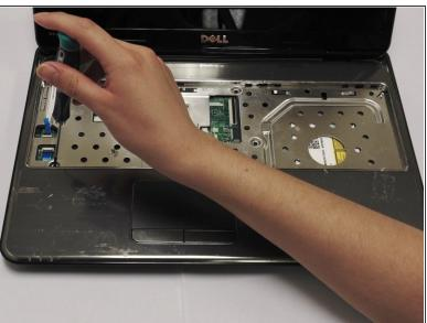
Turn laptop over and open it. Locate and remove the five palm rest screws.
