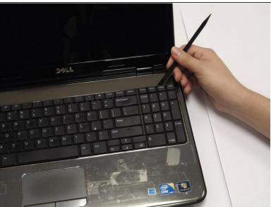
Place your spudger between the keyboard lining behind the x icon and Home keys and pull up.
