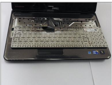
Carefully pull and turn the keyboard over.
