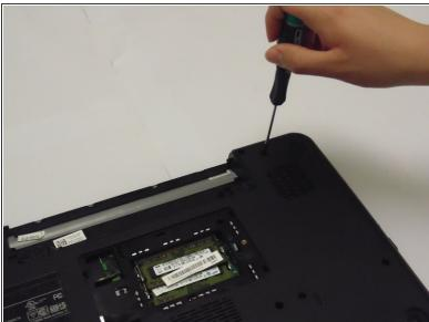
Locate and remove the bottom hinge screws.
