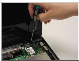
Remove the two hinge screws on both the left and right hand side.
