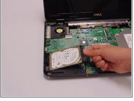
Lift and remove the hard drive.
