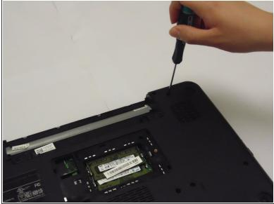
Locate and remove the bottom hinge screws.
