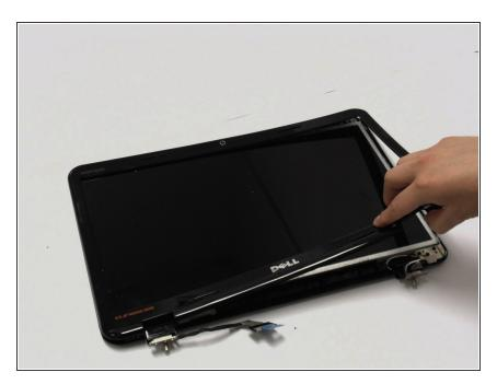
Unsnap and lift the display bezel around the edges and remove it.
