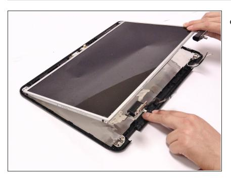
Lift and remove the LCD screen from the backing.
