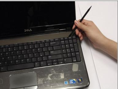
Place your spudger between the keyboard lining behind the x icon and Home keys and pull up.
