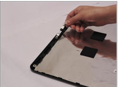
Locate and remove the webcam.
