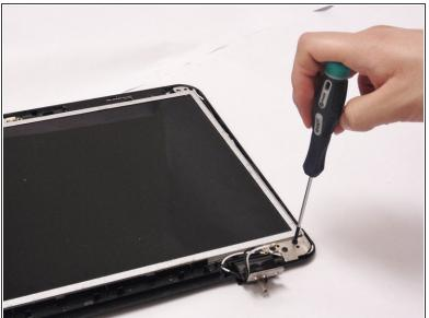
Locate and remove the eight LCD screws outlined in red.
