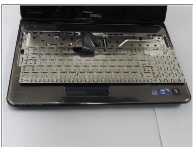
Carefully pull and turn the keyboard over.
