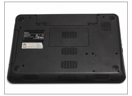
Turn the device over and locate the battery.
