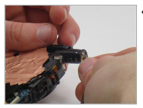
• Pull back on the case, then pull the entire tab out from the case.
