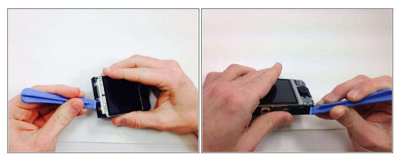
Use a plastic opening tool to gently release the two indicated tabs.
