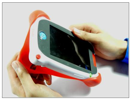
Remove the red rubber case from the device. This should come off with ease.
