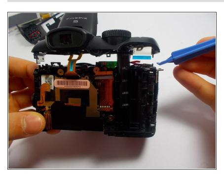
Use the opening tool to pry the top plate off of the top of the camera.
