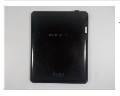
Remove the back plate and place it to the side.
