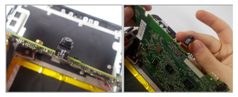
• Gently pull the camera optic fiber out of it's slot to release the flap. This will allow the flap to open easily.
