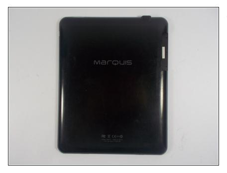
• Remove the back plate and place it to the side of the device.
