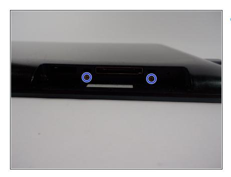
• Using the PH #00 Phillips head screwdriver, unscrew the two screws.
