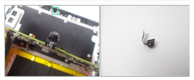
• Last, Insert the new camera into the pinhole camera slot.
