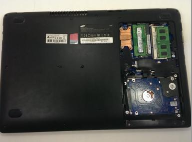
Remove the panel by sliding it down and lifting it away from the computer, exposing the RAM and hard drive.
