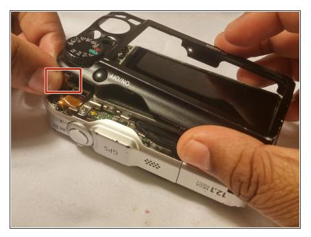
Pull off the back casing and carefully pull the ribbon cable that connects the mode dial and the motherboard using your fingers.
