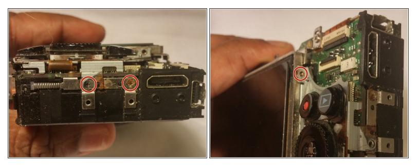
Remove the two 2.5 mm screws that secures the camera buttons to the camera located on the right side of the camera. Then, remove the screw located on the side of the screen. Now, locate the screw under the LCD screen and remove it.
