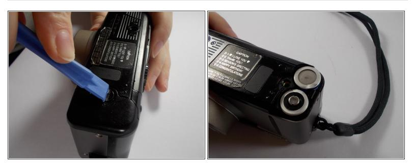
In this step, you will be opening the battery compartment. You can use a plastic opening tool, flathead screwdriver, or any other tool that is similar. On the device there is the word "open" with an arrow pointing in the direction to open the battery compartment.
