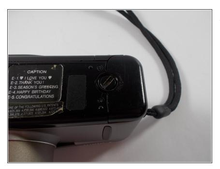
• This area is where the batteries are located, right corner of the camera.
