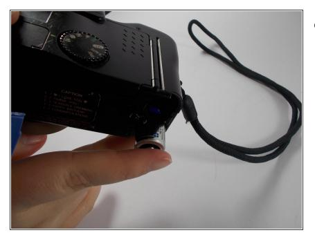
In this step you will remove the batteries. If you tip the camera so it horizontal the batteries will simply fall out, which is much simpler than trying to pick them out of the compartment.
