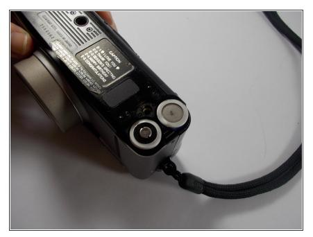
In this step you will add new 3V batteries. You need to make sure they are in the right charge (+,-) port which is labeled when you look inside the battery compartment with a positive and negative sign (positive side of the batter has a little lip negative side is completely flat).
