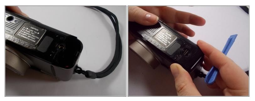
Now that the new batteries are in you can put the cover on top and screw back on the top cover.
