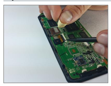
Peel the bottom part of the masking tape off to reveal the ribbon connector.
