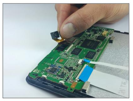
• Pull both camera lenses out of the ribbon connector.
