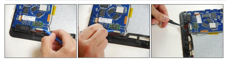
• Disconnect the sliding zero insertion force (ZIF). Use the plastic opening tool or a fingernail to slide the tab out, then pull the cable out.
