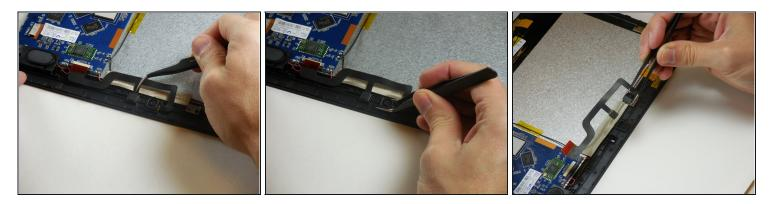
• Pull the cameras out of their resting places in a straight upward motion.
