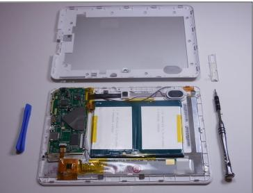
• Once you've moved around the whole device with the plastic opening tool, the back plate will completely release from the rest of the device.
