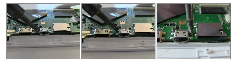
• Work the iron on one prong at a time that is soldered to the motherboard. The USB port will release from the motherboard.
