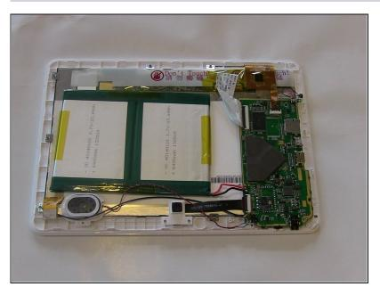
The battery rests flat on the inside surface of the tablet. It is a rectangular shape and has blue and yellow tape.
