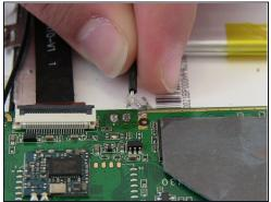
• Once both wires have been desoldered, remove the battery from the device.
