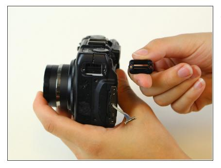
• Remove the current bar and insert its replacement.
