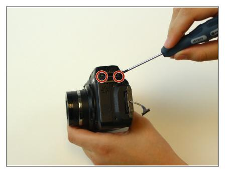
• There is one screw on the left and right sides of the retaining bar. Using a Phillips-head #00, unscrew each.
