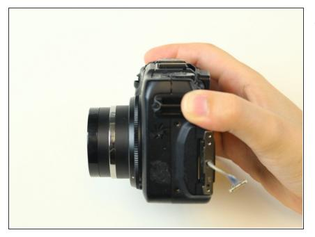
Hold the camera so the retaining bar is visible.
