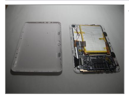
Remove the back cover with your hands once all points have been unlatched. It should separate completely from the screen that contains the battery and chip components.
