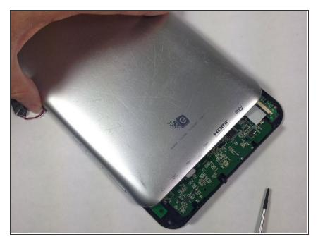
Slide the rear panel away from the base parallel to the screen.
