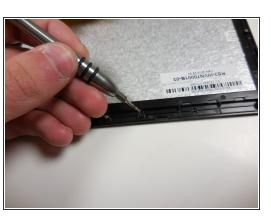
Remove all 14 of the 3.6mm screws using a PH00 screwdriver.
