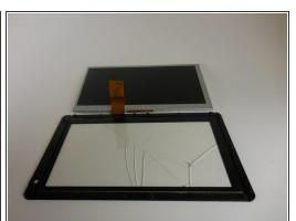
• Remove the grey monitor from the glass screen cover by gently lifting it up.
