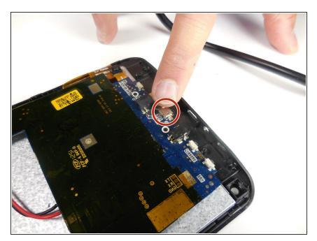
The charger port is located on the underside of the motherboard (as pictured).
