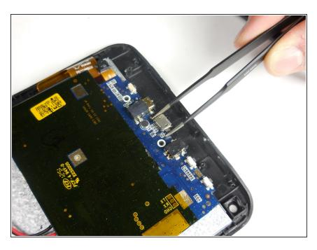
Remove the charger port by using tweezers and gently pulling.
