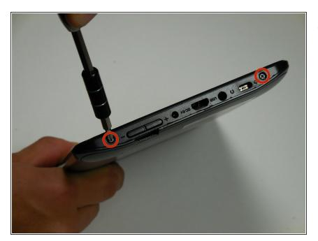
Remove the two 2cm screws on the bottom using the PH0 Phillips head screw driver.
