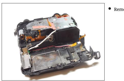
• Remove the back casing.
