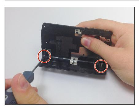
Re-screw the two silver screws tightly back into the silver plates.
