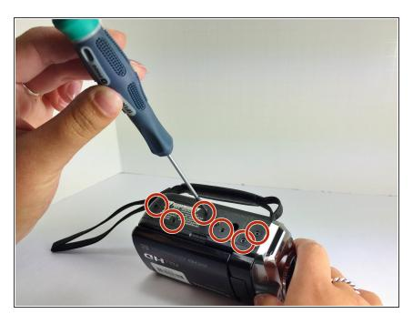
Unscrew the six .5 mm Phillips #00 screws on the bottom of the camcorder.
