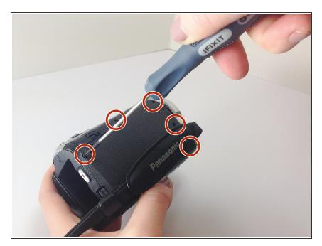
Using the Phillips #00 Screwdriver, unscrew the five .5 mm Phillips #00 screws on the hand-strap side of the camcorder.
