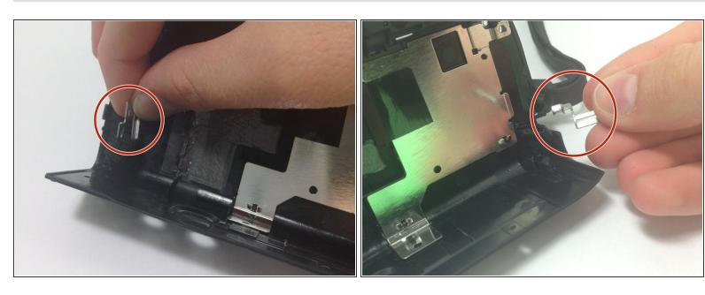
Remove the two silver plates from the loops of the hand-strap.
