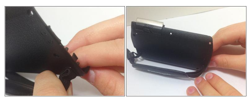
Feed the larger loop through the hole in the opposite corner of the side cover.
