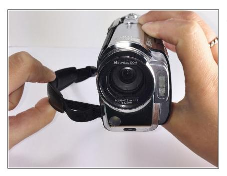
When the side cover is securely fastened, you have completed the hand-strap replacement of your Panasonic HDC-TM15 camcorder.
