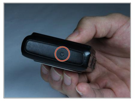
• Remove the 5.0 mm screw on the left with a Phillips #00 screwdriver.
