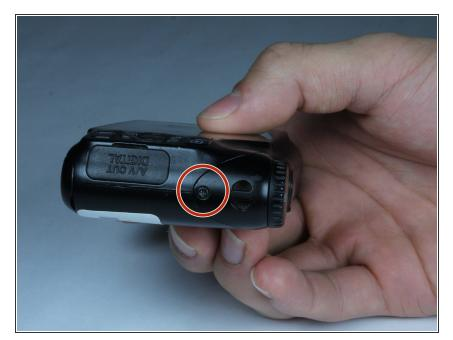
Remove the 5.0 mm black screw on the right with a Phillips #00 screwdriver.
