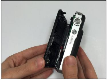
• Separate the front piece of the camera from the back, revealing the motherboard.
