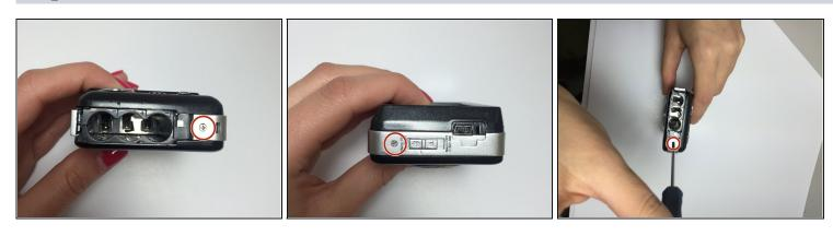
Use a Phillips #00 screwdriver to remove the 3 mm screws at the sides of the camera.
