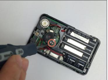
• Use a Phillips #000 screwdriver to remove the two 2.3 mm screws that surround the lens.
