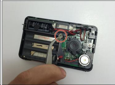
Remove the two silver plates using tweezers.
