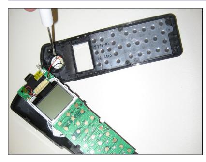
• Gently lift out speaker using a small flathead screwdriver.
