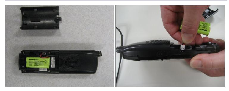
• To remove the battery, gently pull up on the white connector located on the left side of the phone.
