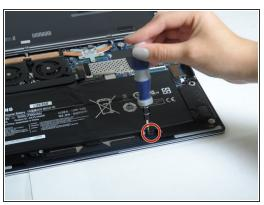
Unscrew the four 4.55 mm Phillips #000 screws on the edges of the battery.
