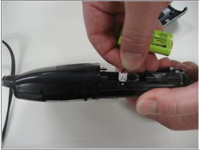
• To remove the battery, gently pull up on the white connector located on the left side of the phone.
