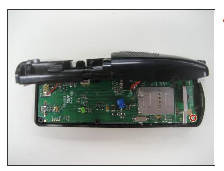
Using a small Phillips head screwdriver, remove the single screw (located at the top right) holding the circuit board in place.
