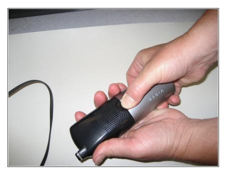
Place your thumb in the groove on the back of handset. Next, push down with your thumb and then slide the battery cover towards the bottom of the phone to remove the battery cover.
