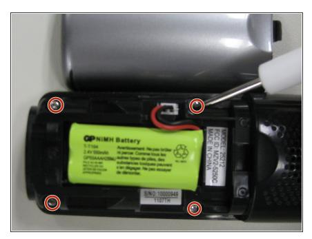
Remove the four screws, located at each of the corners within the back encasing, with a small Phillips head screwdriver.
