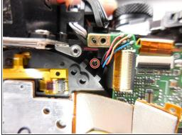
To get the lens assembly out, you need to remove four 6mm PH00 Philips screws
