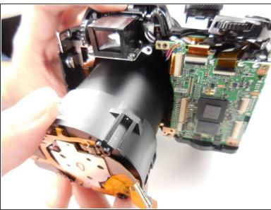
With the support screws out, you can simply slide the assembly out of the casing.
