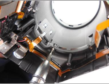
Remove five PH00 Philips screws with a Philips screwdriver.
