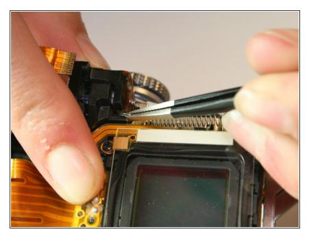
Using tweezers grasp the end opposite the screw, pull against the tension and twist the spring out. You may have to try it a couple times, but just keep twisting and pulling at the spring.
