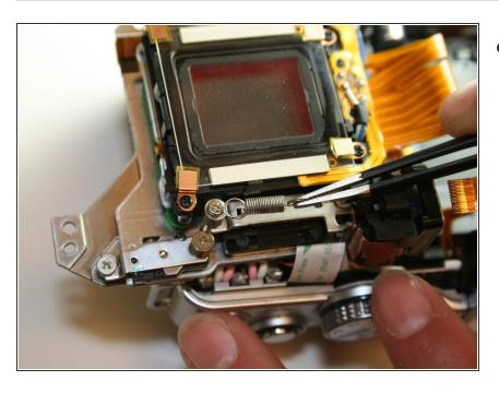
When you pull the spring off one side, it will easily come off the other side. Just slide the spring off.
