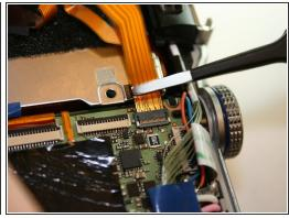
Unlike previous connectors, this cable has a light grey clip holding it in place on opposite side of the connector in regards where the ribbon is inserted. Flip it up and then using your fingers, gently pull the top ribbon cable out.
