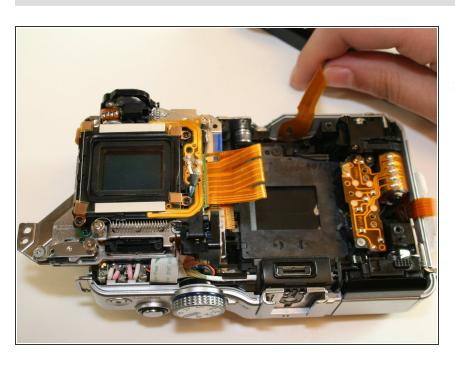
The sensor assembly has been removed.
