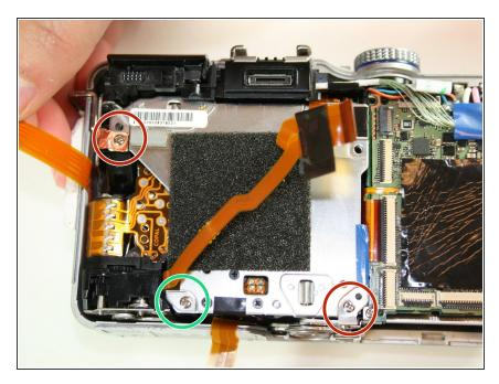
Using a #000 Phillips screwdriver, remove the 6.0 mm screw on the bottom left hand corner. You can locate the screw on the picture as the green circle.
