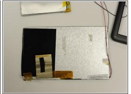
Remove the battery by using the spudger to gently pry the battery away from metal case around the front screen.
