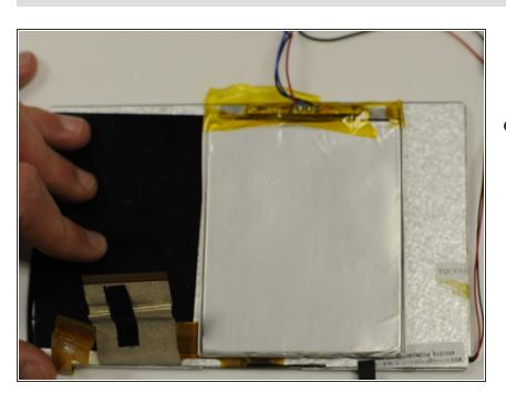
Remove the motherboard by gently pulling it away from the bottom of the device. To reassemble your device, follow these instructions in reverse order.
