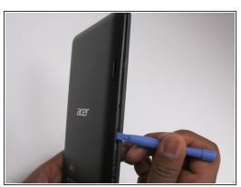
• Insert a plastic opening tool into a gap near the charging port at the top of the device. Slide the tool in either direction along the device.
