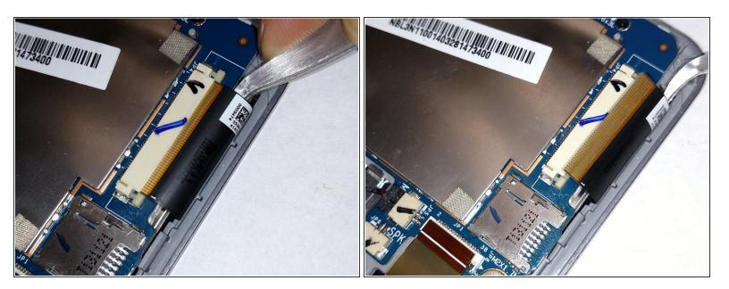
Use tweezers to gently remove black ribbon from locking mechanism.
