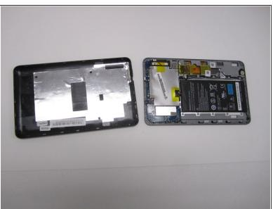
Once all the sides have been separated, you should be able to simply lift the cover off of the device.
