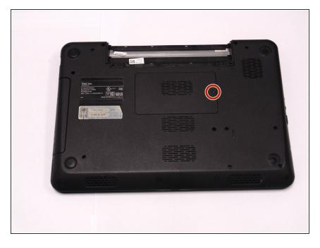
Locate the RAM compartment on the device and locate the screw on the right hand side.
