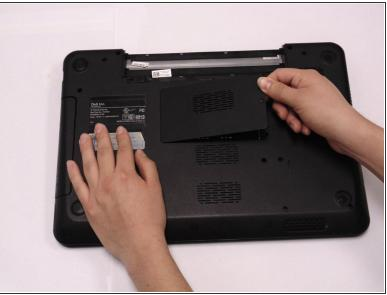
Take your screwdriver and loosen the screw. Then remove the cover.
