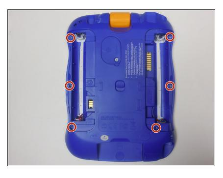
Remove the six 7.6mm screws found in the battery compartment using a PH00 screwdriver.
