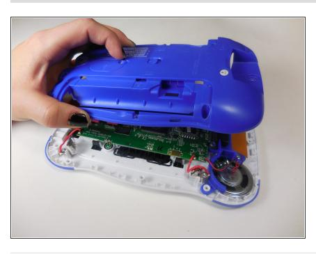
Carefully separate the back panel from the front panel revealing the motherboard connected to the front panel.
