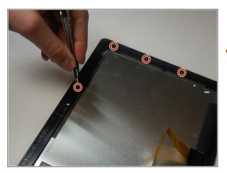
Using the PH00 screwdriver unscrew and rotate the plastic tabs that are holding the screen in place.
