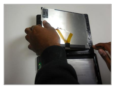
• Remove the screen from the device.
