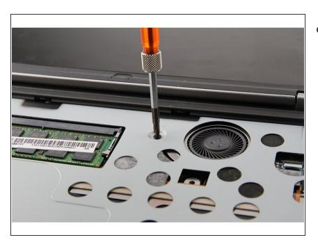
Remove the two screws securing the midframe.
