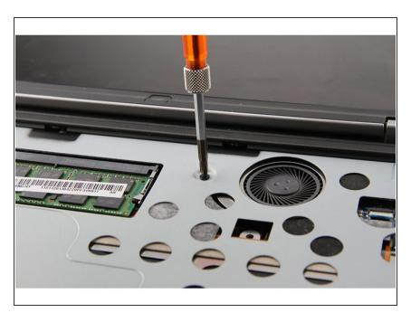
Remove the two screws securing the midframe.
