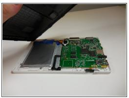
Use your fingers to remove the rest of the back. Slowly apply pressure from each side to detach each clip connection.
