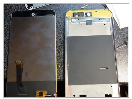
Put some adhesive (or some glue?) I used thin double-sided tape I had cut the right shape. the side of the screen are less than 1mm wide, it's hard to do here...
