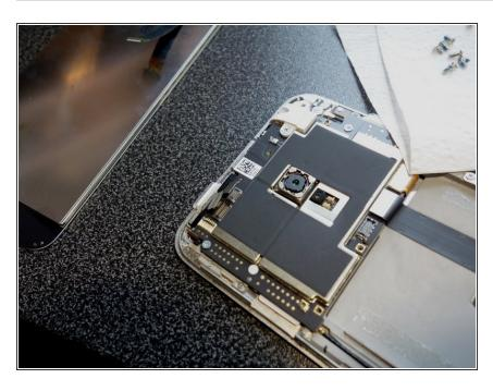
• Unplug all the connectors to the motherboard, included the two antennas The small flat ribbon in the corner is a little tricky, you have to switch the black part of the connector, not the white one like some other similar I saw before.
