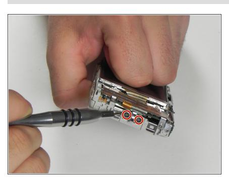
Remove 2-2.90mm using a #000 Phillips screwdriver.
