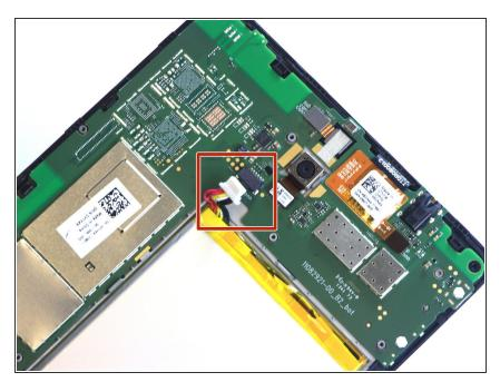
Unclip the power clip from the motherboard by pulling down gently towards the bottom of the tablet.
