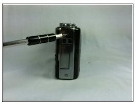
Replace the side panels and replace the four screws to secure the side panels.
