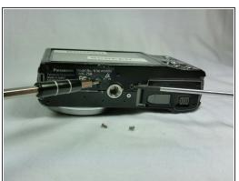
Replace the front panel and install the screws on the bottom side of the camera.
