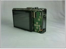
Reconnect the new screen wiring into the motherboard as shown in the picture. Replace the new screen into the mounting bracket.
