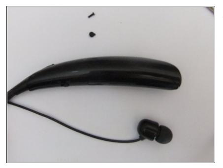
Once the new magnet is in place, the casing can be pushed back together.
