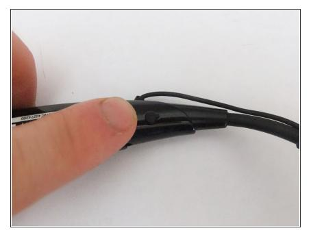
• Push the small rubber piece back into place over the screw.
