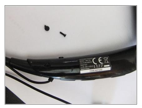
Remove the small screw from the underside of the device and place it aside.
