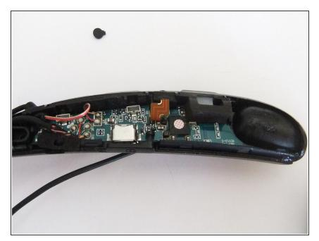
Once the case is open, the small magnet is now visible and can be replaced.
