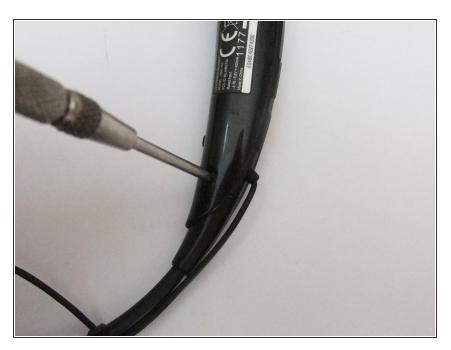
The small screw that was taken out at the beginning can be screwed back into the device.
