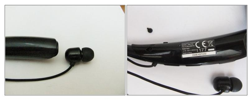
• Find the side of the device with the defective magnet. Remove the rubber piece on the underside of the device that protects the screw.
