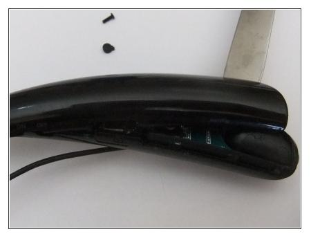
Place a small prying tool in between the two cases and slowly push the two apart. Be sure not to force the case apart, as it may snap in the process.
