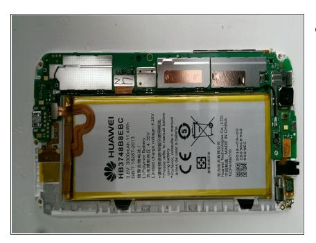
The disassembled smartphone with the aluminum back removed
