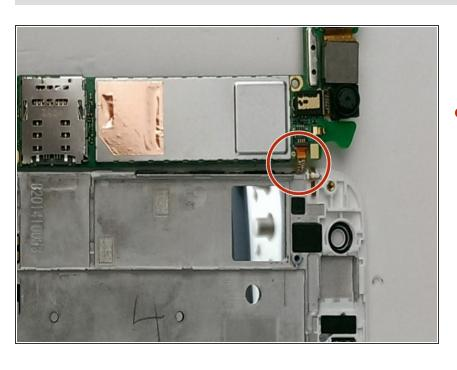
Gently rotate outside the motherboard, making sure not to break the little indicated connector
