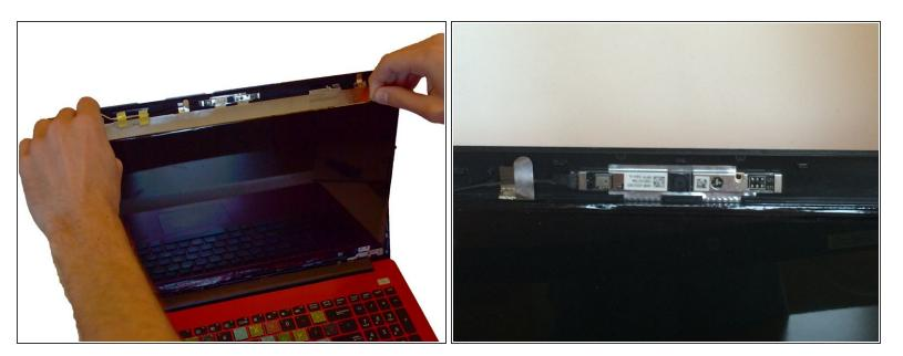
• Carefully pull the top of the monitor cover off with bottom still attached, and view the webcam attached by a wire.
