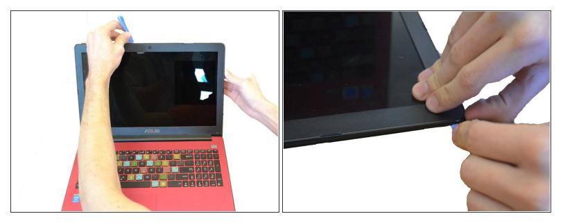
Remove the trim from the top of the monitor by using the Plastic Opening Tool to carefully pop off the clips around the parameter.
