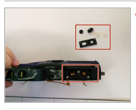
Replace the shutter/power button or button component.
