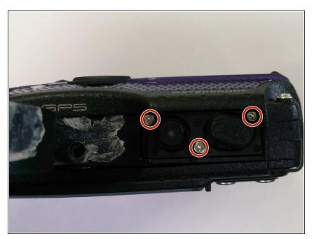
Remove the 3, 2 mm screws under the rubber buttons.
