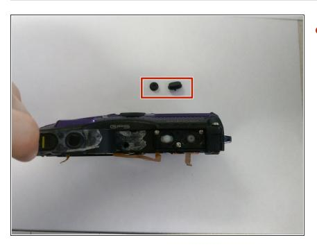
Using tweezers pull straight up to remove the 2 rubber button toppers
