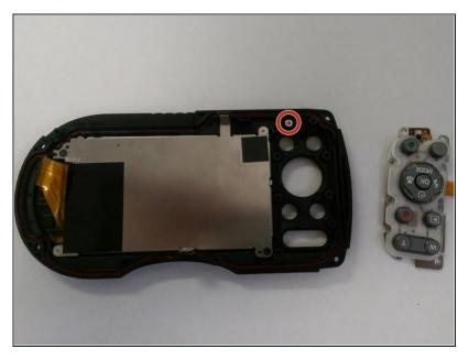
• Remove the 1, 2 mm screw near the edge of the device.
